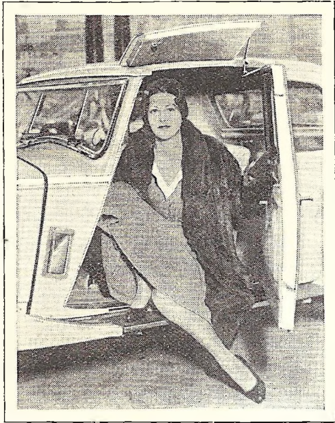
This new British made auto is equipped with automatic trap door in the roof to prevent bumping the head. The hinged part swings upward with opening of car door.
