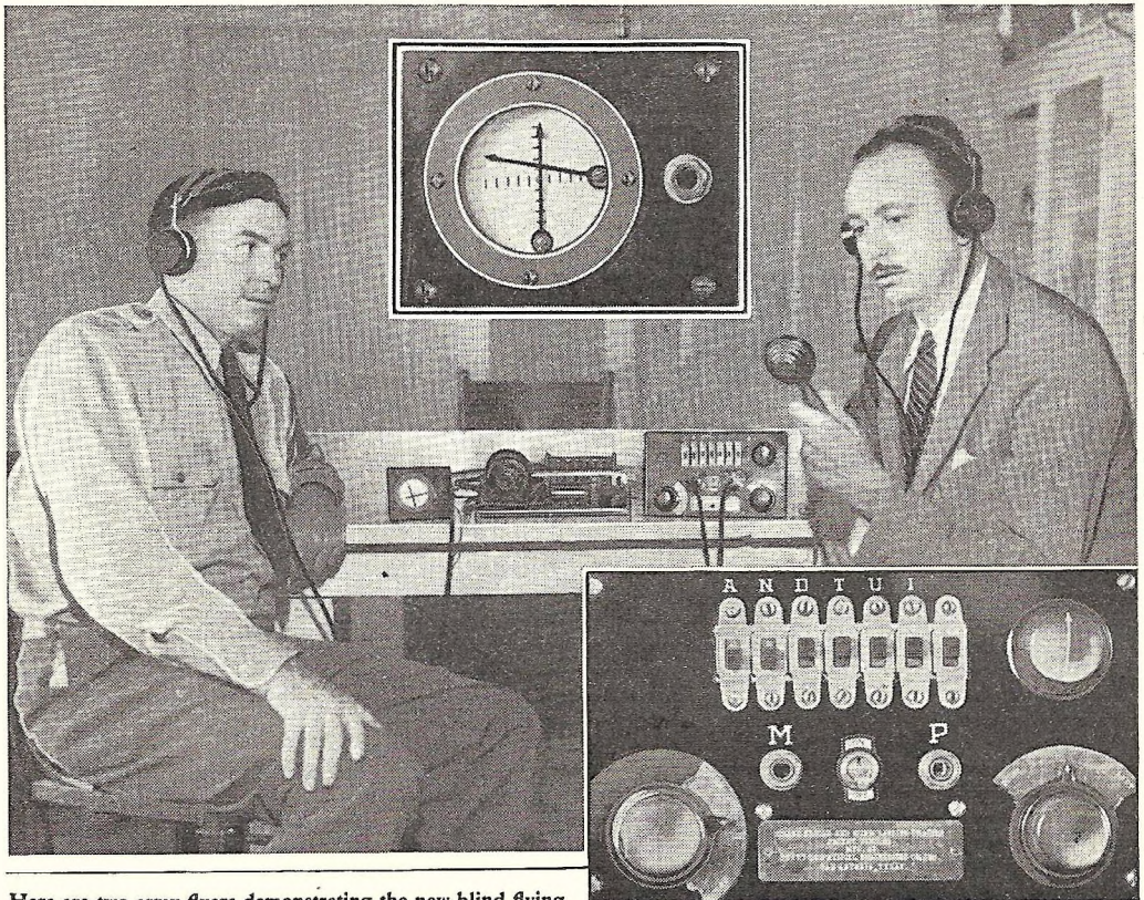
Here are two army flyers demonstrating the new blind flying instruments. Student (at left) watches dial shown in inset to learn whether he's off course. Instructor at right operates control dial (shown below) to show student direction ship is flying with relation to landing field. Instructions are given through the mike—Photos courtesy U. S. Army Air Corps.
