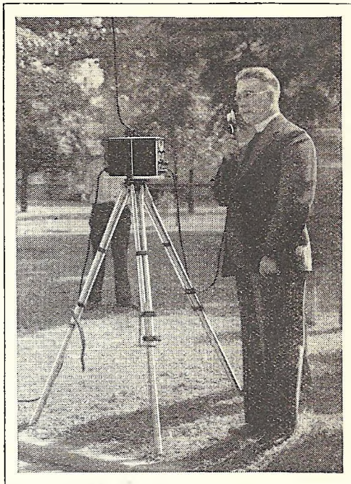
Here's the new "transceiver" set up ready for operation. Mounted on tripod, outfit weighs 22 lbs. and proves ideal for police work, fire fighting and tunnel disaster rescue jobs.
